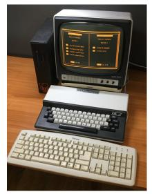
It has been a common problem with older Microbee computers that keys on the keyboard become non-functional. With no supply of original switches, people have to resort to removing them, taking them apart & attempting repairs with varying levels of success.
