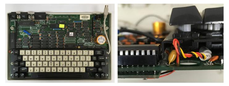
Next, on the underside of the baseboard, with the tinned copper wire provided, solder 20mm lengths to each of the corner pins of IC1 (the CRT controller) - pins 1, 20, 21 & 40. Also, pins 3, 8, 9, 10, 11, 12 & 13. Note though, that if you have taken Option 3 (no track cut) in the track cut section above, please leave out the wire that would normally be soldered to Pin 3 of the CRT controller socket.
